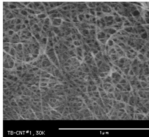
*Figure 2: SEM Micrograph of CNT Film at  $100\ \Omega/\square$*
