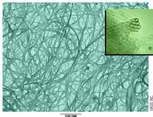
**Figure 1** Graphite sheets can form carbon nanotubes (inset), which can combine, in turn, to form ropes. Applied as very thin films, they create a fabric of nanotube ropes that can conduct electricity in circuits (main image).
