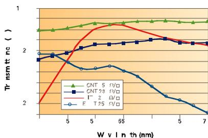
**Figure 3** Curves of optical transmittance versus wavelength for different grades of carbon nanotubes and ITO show relatively flat transmittance for nanotubes across the visible spectral region. All transmittance values refer to the transparent conductor layer only, with substrate effect removed.
