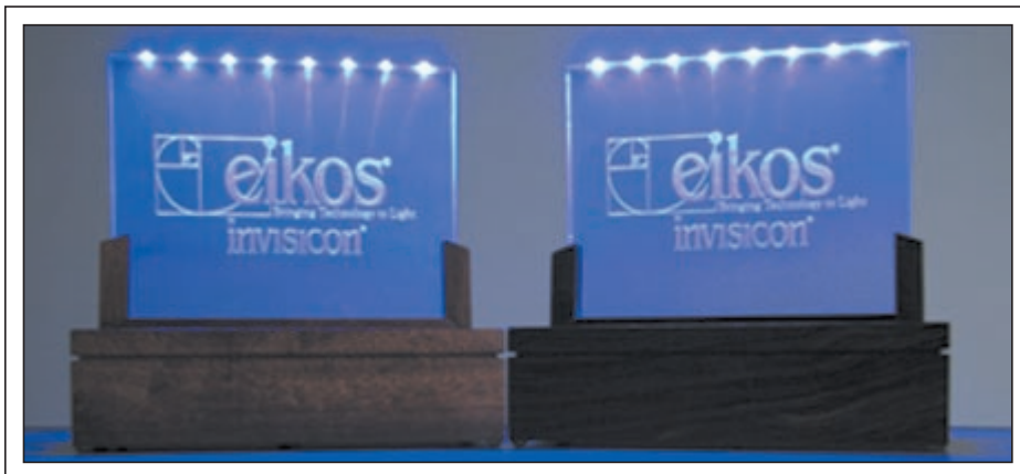
Fig. 4: Transparent SWNT electrodes in LED-illuminated displays.
