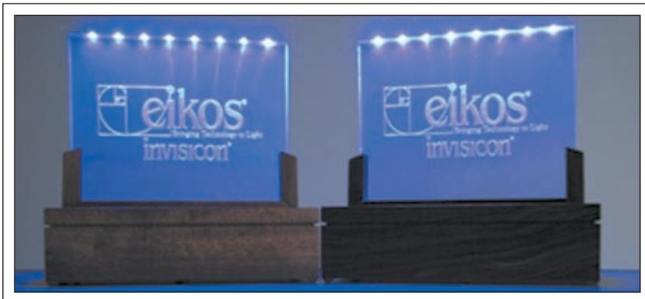
**Fig. 4:** Transparent SWNT electrodes in LED-illuminated displays.
